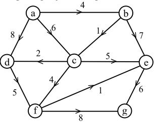
Obtain the shortest distance matrix between all the vertices using Floyd-Warshall algorithm.
